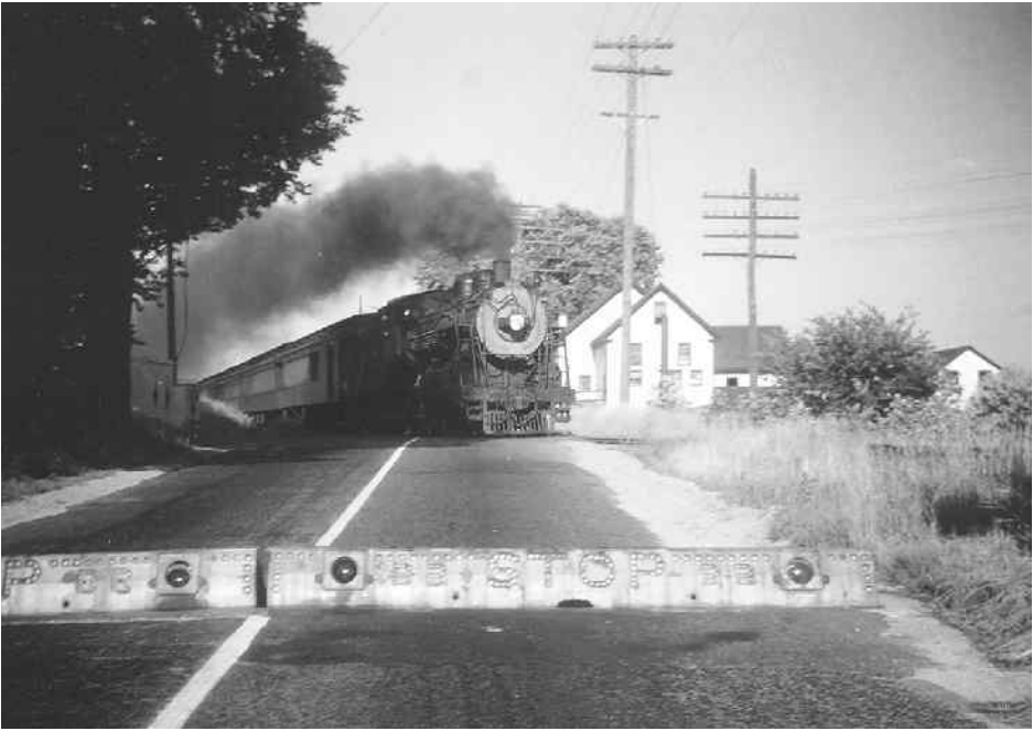
A gaudy nine-inch-high steel barrier rises from under the ground to keep cars away from a train in July 1947. (Photo by Donald S. Robinson)
